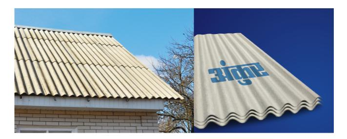
**Ankur Fibre Cement Corrugated Sheets** are manufactured using a homogeneous mix of Ordinary Portland Cement and fly ash with high strength reinforcement provided by fibre and cotton pulp. The sheets are manufactured at our state-of-the-art, fully automatic plant using the Mazza Process.
